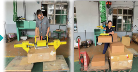
Vacuum Lifter for Labor-saving Handling
